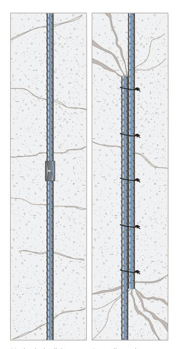
Mechanical splicing provides the assurance of maintaining load path continuity of the structural reinforcement independent of the condition or existence of the concrete
