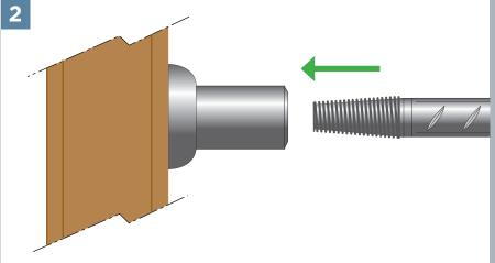
To make the joint bring the tapered threaded continuation bar and the welded coupler together.
