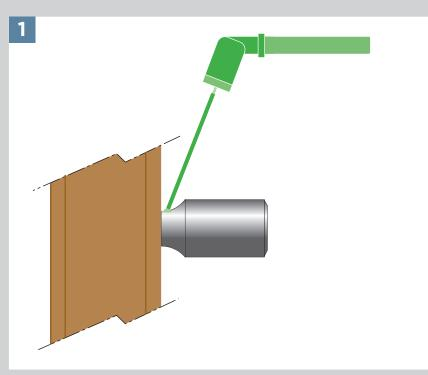
The C15N coupler is welded to the steel structure prior to making the joint.
