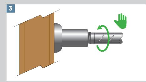
Screw the taper threaded continuation bar by hand into the coupler.
