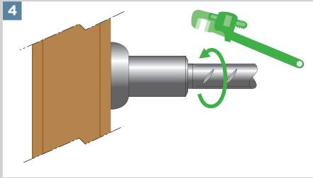
Tighten the joint with a LENTON wrench to the correct torque as specified in the installation manual.
