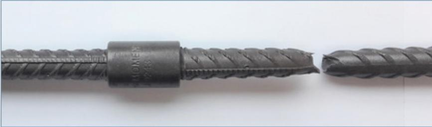
Ancon BT Type A Couplers have been tested to satisfy the requirements of CARES Appendix TA1-F for Couplers with reinforcing bars to BS4449 Grade B500B as appropriate. The testing comprised the following elements:
