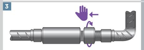
Set the bent bar to the required position then screw the Lock Ring by hand towards the coupler body.
