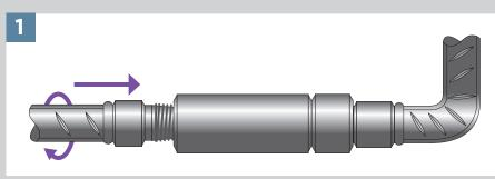
To make the joint bring the two components together.
