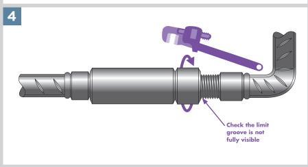
Tighten the Lock Ring fully against the coupler body with a LENTON wrench to the correct torque as mentioned in the installation manual and on the wrench itself.
