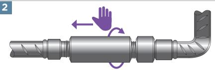
The Coupler Sleeve is then screwed out by hand to engage the Male Taper Stud threads and is tightened to the correct torque as described in the LENTON installation manual.
