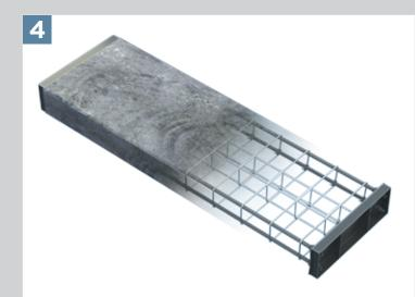
The fabricated reinforcement cage is then placed on the casting bed
