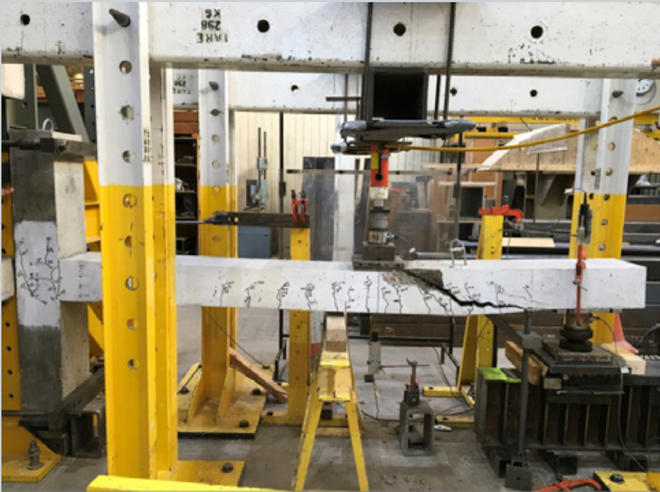
Figure 1 - Test arrangement and failure mode in shear
